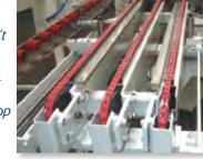
designing with PowerTwist Friction Top from the start, they were able to produce systems that rarely require maintenance to the belts, but can be done in minutes if the need does arise.
