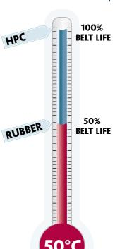
Fenner Drives HPC V-Belts are different in two significant ways. First, they are made of custom reinforced polyurethane elastomers with excellent resistance to high operating temperatures. Second, the unique link design results in belt constructions which limit flex induced heat build-up; a greater surface area also dissipates any heat generated more effectively as compared to a solid construction rubber V-belt... a lower internal belt temperature = a longer belt life.
